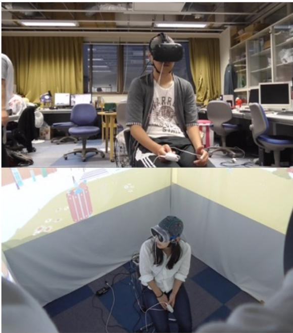
Fig.1 (Upper) HMD and (lower) SCREEN-GOGGLE, which restricts the vision of the user by applying goggles.
